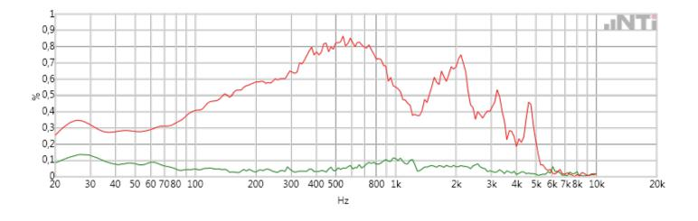
THD Measurement curve, THD @ 110 dB/SPL, @ 1kHz Green = 7mm Sennheiser True Response® transducer, FA 500 Custom Red = 6 balanced armature, 3-way In-ear monitor Equipment: Coupler / Ear simulator: GRAS RA0402
